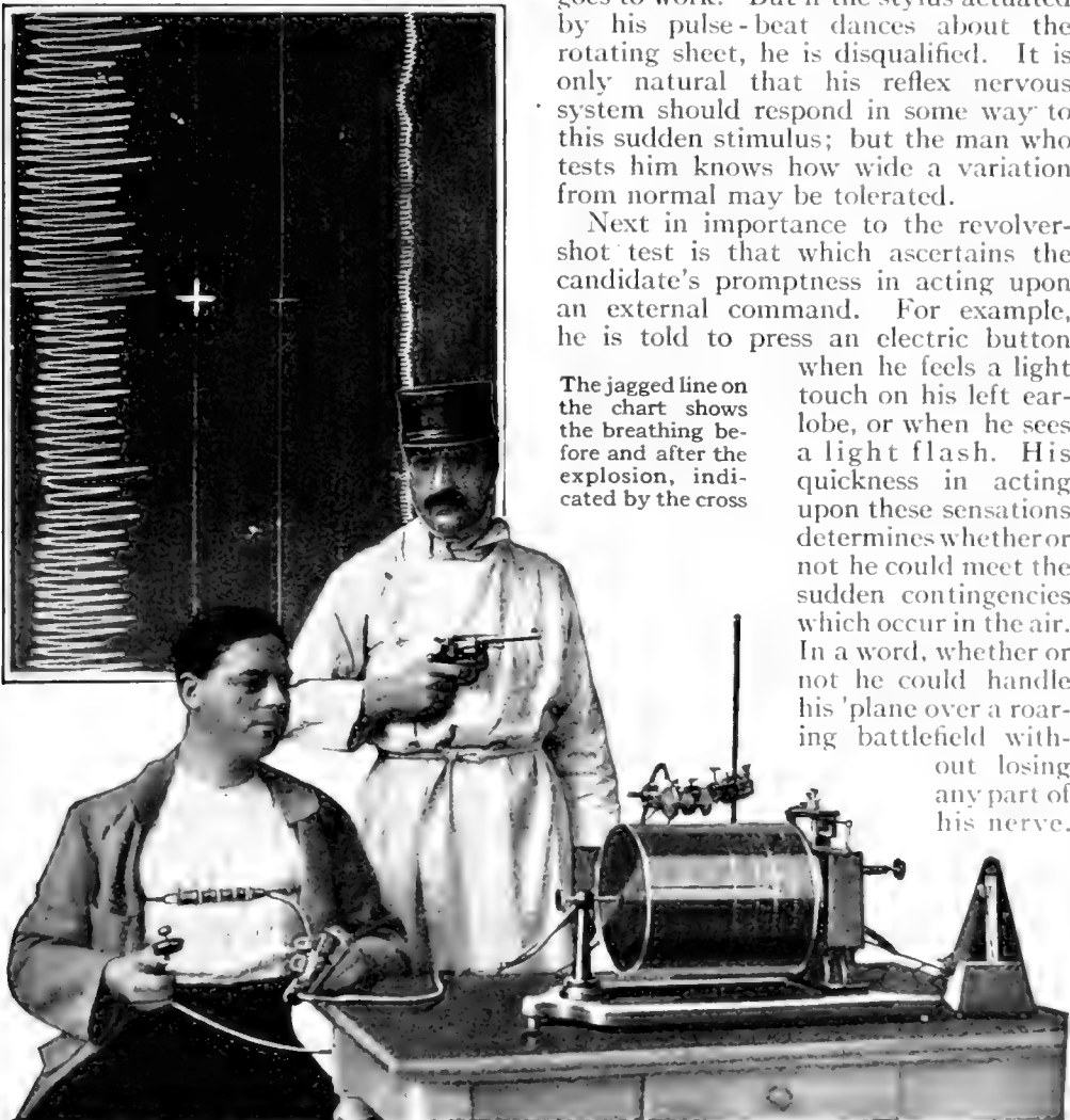
The d'Arsonval chronometer which records on a smoked paper cylinder the pulse beats, respiration and nervous tremors of the applicant when a pistol is fired behind him
